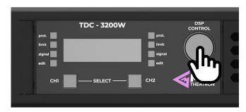
Pressing any of the Channel select buttons opens the Channel menu for that channel.
