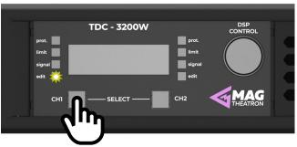
If both CH1 and CH2 buttons are pressed at the sametime, both channels will be edited simultaneously with identical parameters.
