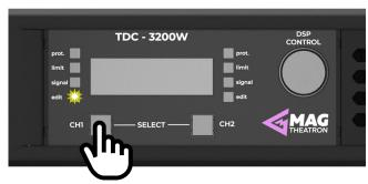
Pressing both Channel buttons at the same time opens a Channel menu for controlling the parameters of both channels at the same time.
