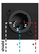
Loudspeaker connection, stereo mode
