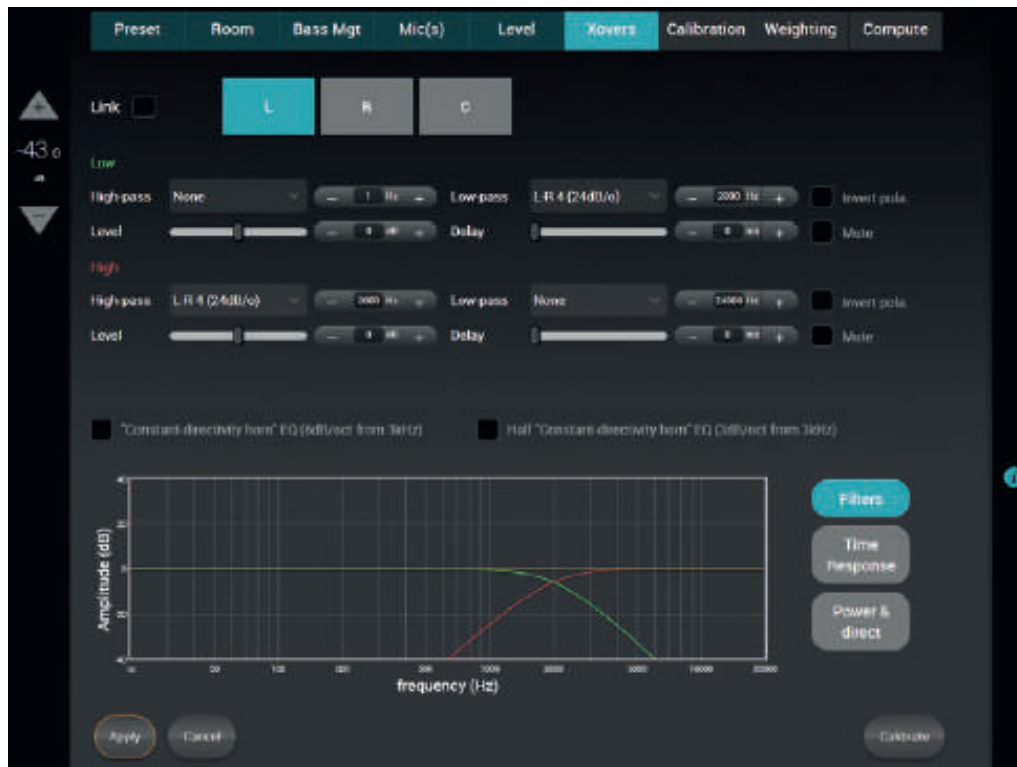
Figure 73: Calibrate manually a crossover
