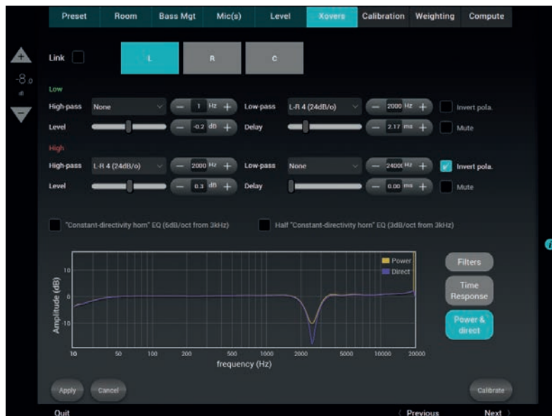
Figure 81: frequency response (power and direct)
